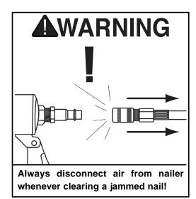
To clear a jammed nail from the discharge area with the Model G6049:
